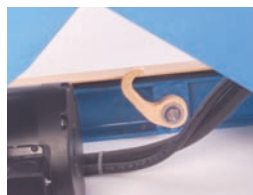
Hinged maintenance catches
