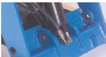
Flow limiting valve provides a controlled descent in the event of a hydraulic line rupture
