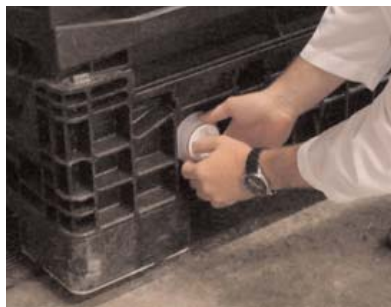
Pull dispense fitment through the dispense chamber and guillotine of the tote.
