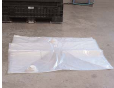
Unfold liner once horizontally and then once vertically. Remove plastic wrap from fitments.
