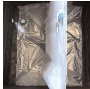
Place four corners of liner into the four corners of the tote.
