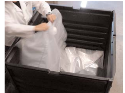
Hold onto the top of the liner where the filling fitment is located.
