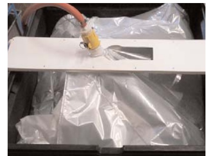
Attach hose and begin filling process.
