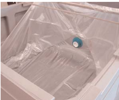
As liner dispenses, continue to wind liner into winder and move toward dispense fitment.
