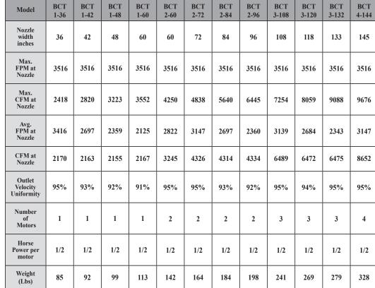
Sound Level: 60 dba / Sound level measured 10 ft.from the unit in a free field based on a one-motor unit.
