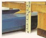
Forks lower to 3.3 in. for optimal clearance under skids.
