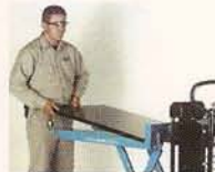
Accessory tables mount on top of the forks.
