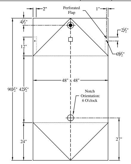
ALL TOLERANCES ARE (+/- 1/2"), DIMENSIONS ARE INSIDE SEAL TO SEAL, SHOWN FILL & DISPENSE UP.
