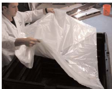
Place liner in tote with dispense fitment end in first.
