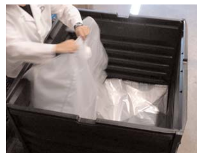
Hold onto the top of the liner where the filling fitment is located.
