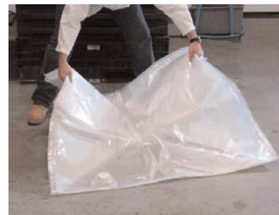
Grab the two back corners so the dispense fitment is towards the front-right of the liner.
