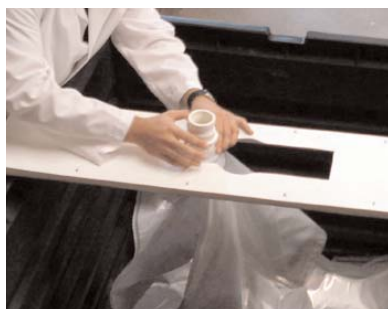
Place fill fitment in fill bridge and attach Cam-lock.
