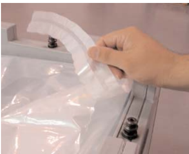
Tear perforated flap from liner.
