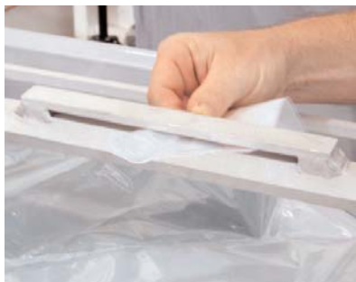
Insert perforated flap into winder.
