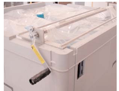
Before dispensing, start winding flaps into winder.
