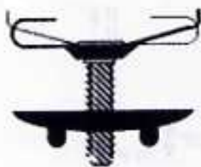
CADDY Clip made of spring steel
