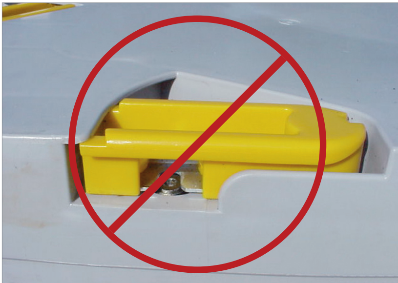
Handle not properly engaged with locking bolt.
