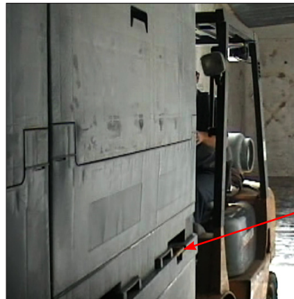
2. Proper stacking with feet and lid interlocked.
