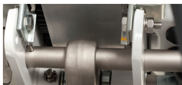
Nickel-Plated Suspension Shaft and Suspender
