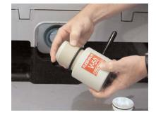
Thread 2" BSP pusher/cutter adapter to V50 gate valve.
