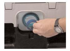
Flip crown cutter 180° and put back into fitment.
