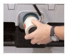
Thread V50 gate valve with pusher/cutter adapter to fitment until it stops.
