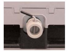
Membrane is now cut, attach necessary adapter.
